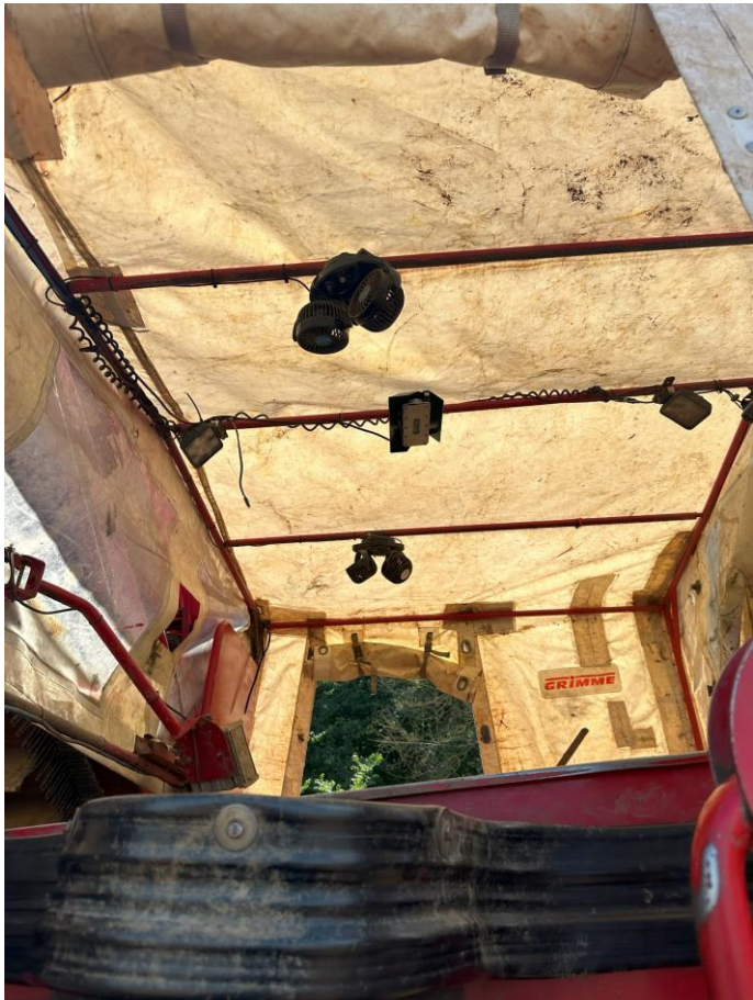
The HarvestEye camera mounted using an 'offset plate' to the central mounting pole within a picking canopy.
