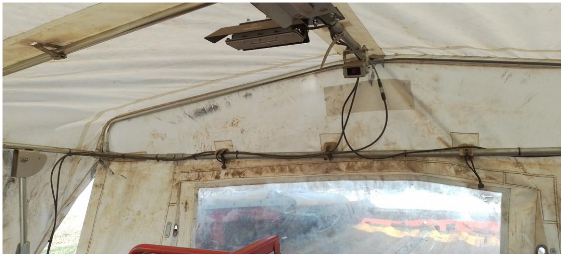
The HarvestEye camera mounted using an 'offset plate' to the central mounting pole within a picking canopy.
