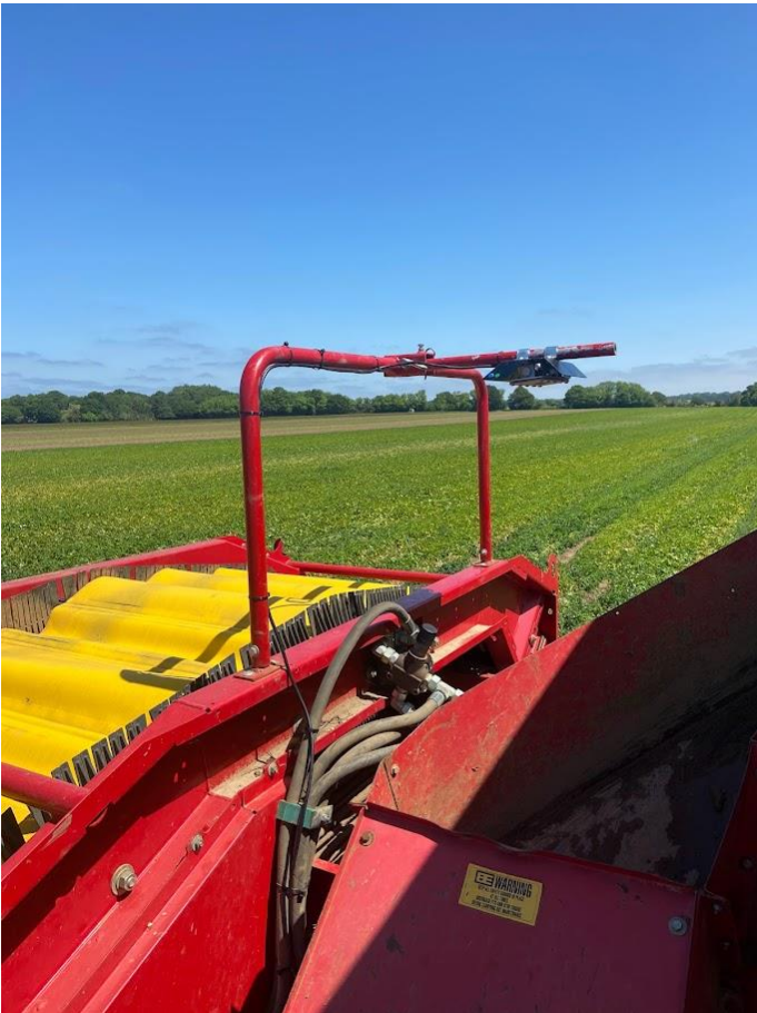
The HarvestEye camera mounted using an 'offset plate' to the central mounting pole within a picking canopy.
